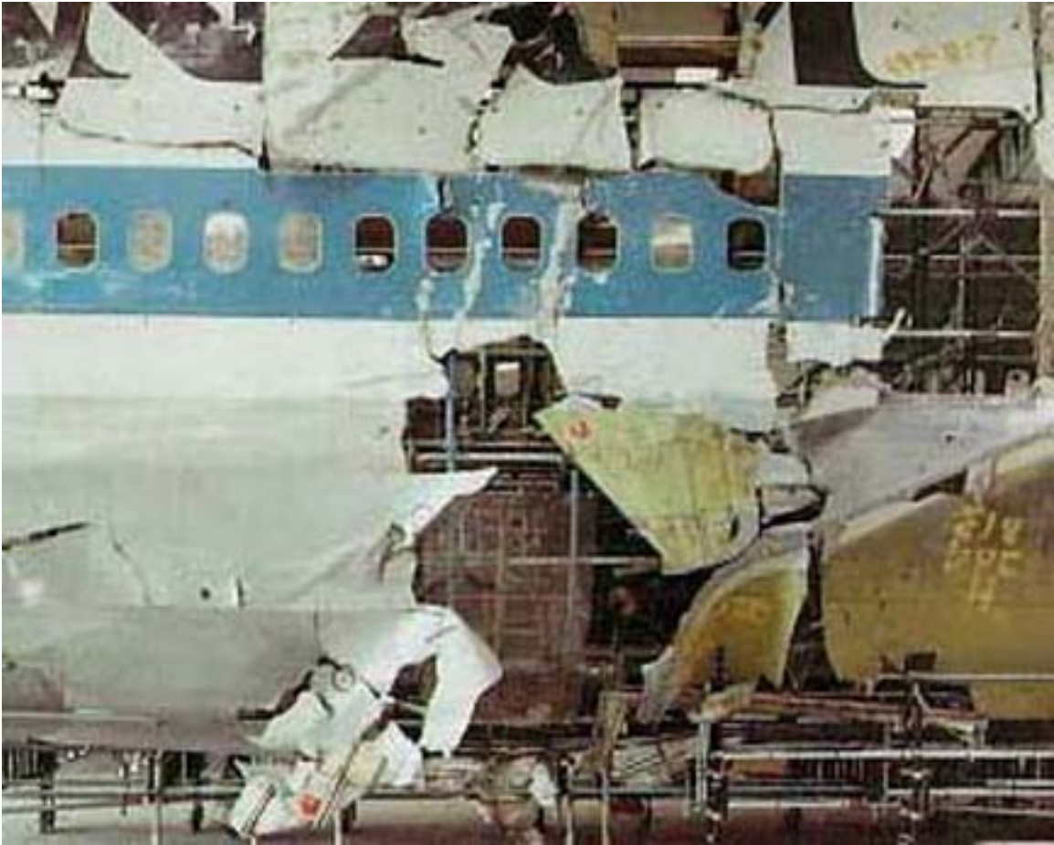
Port side of Pan Am Flight 103 forward of the wing showing the small 'bomb' hole and relatively smooth and intact fuselage skin around it.
