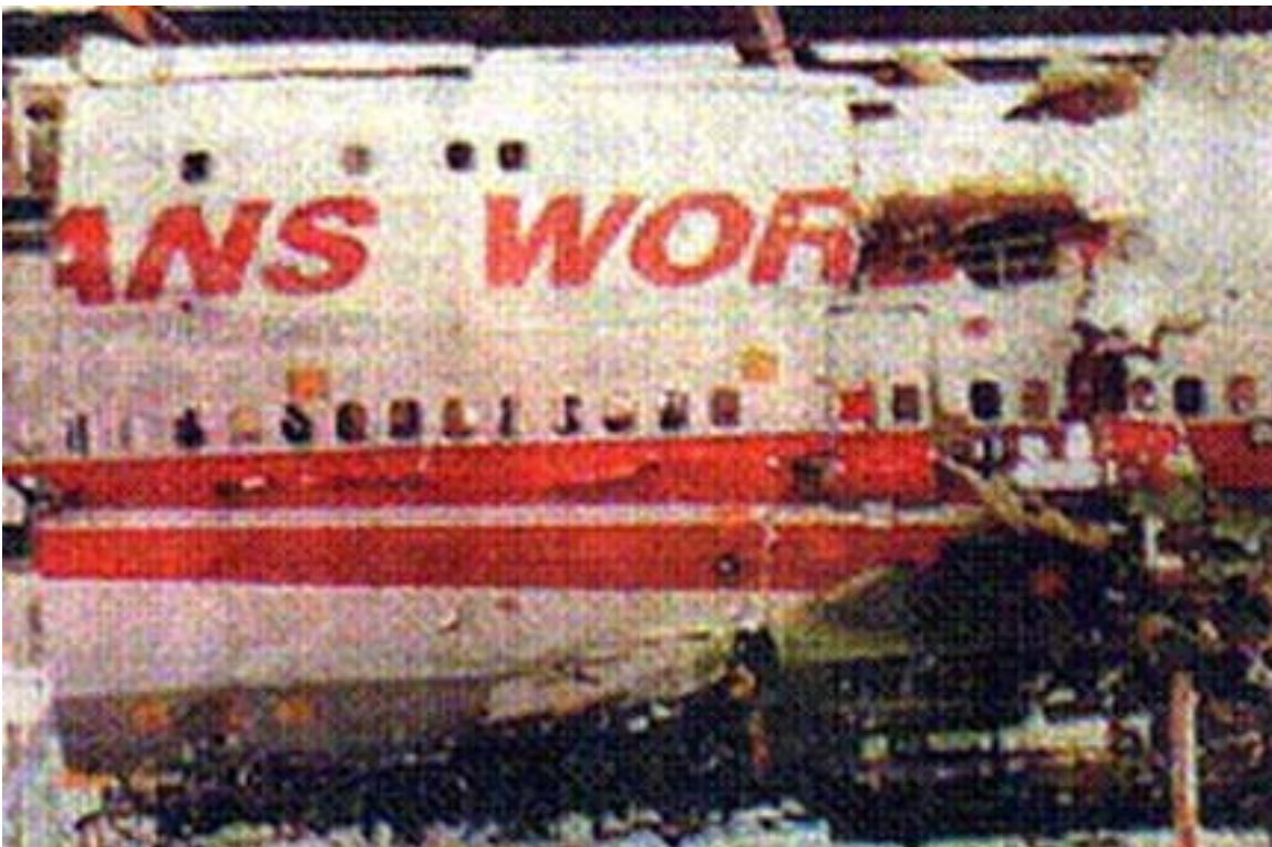
Photograph of the port side of Trans World Airlines Flight 800 showing the relatively undamaged skin forward of the wing, nose to left.
