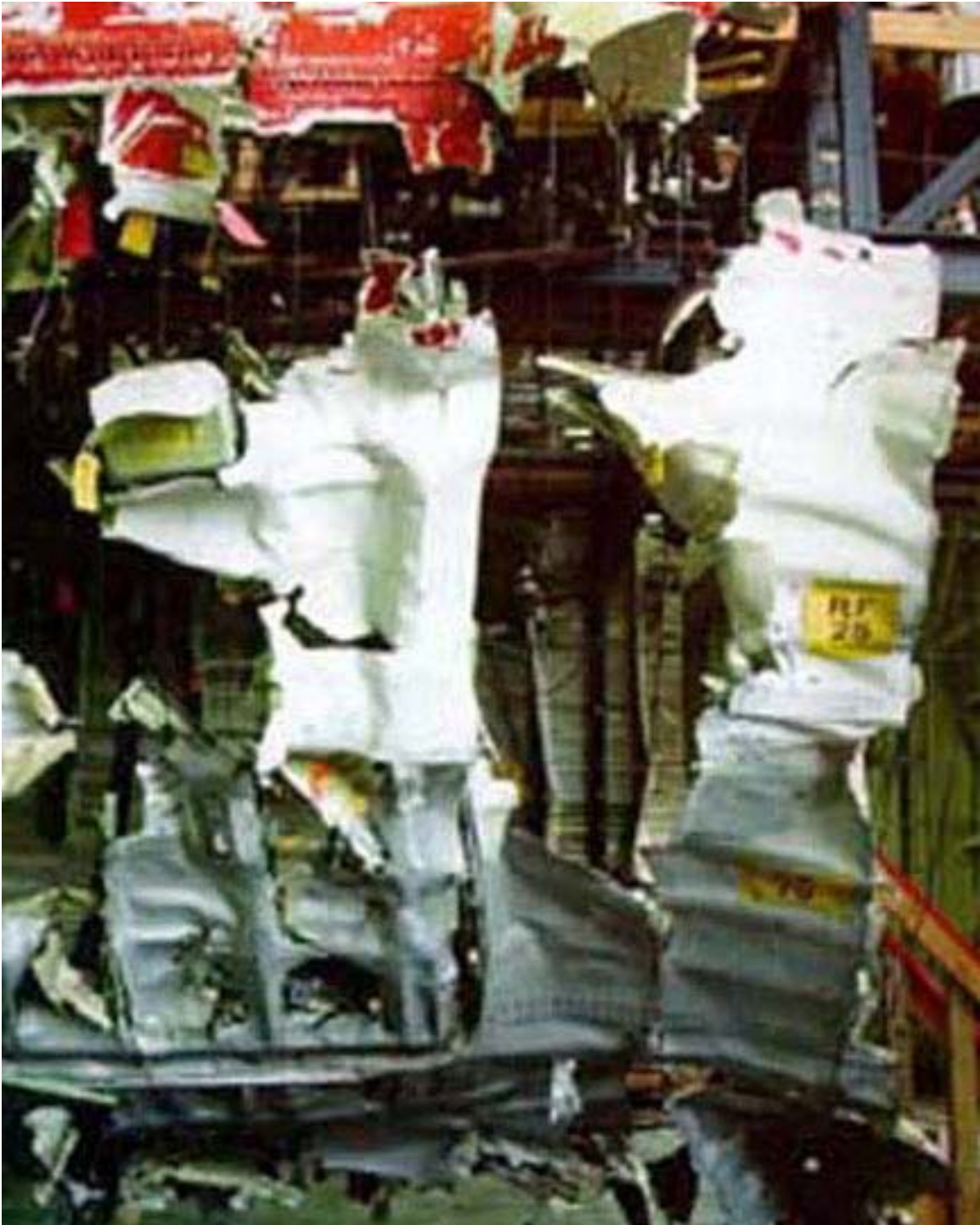
Trans World Airlines Flight 800 Forward cargo door showing separated and replaced forward pressure relief door.
