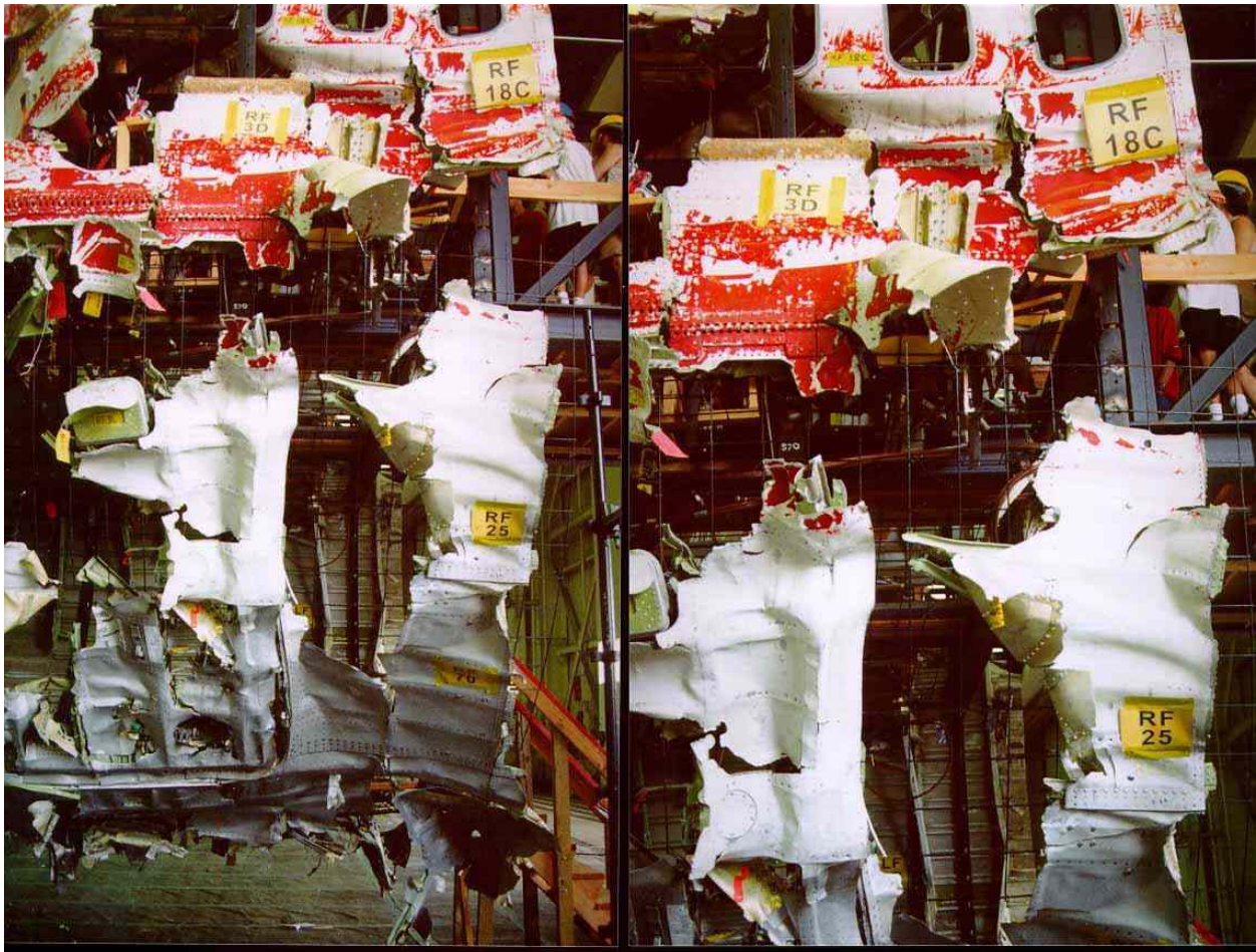
Two pictures of forward cargo door forward midspan latch area right side of aircraft, nose to right revealing outward peeled in petal shape and strange red paint smears.
