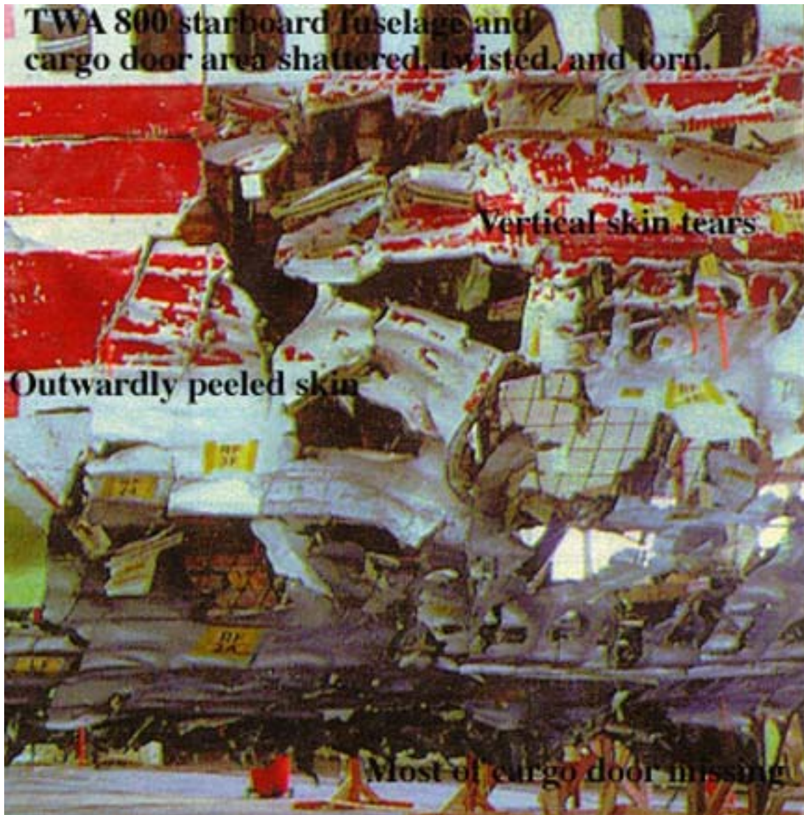
Shattered starboard side around forward cargo door of Trans World Airlines Flight 800 revealing outwardly and petaled shaped skin around aft midspan latch.
