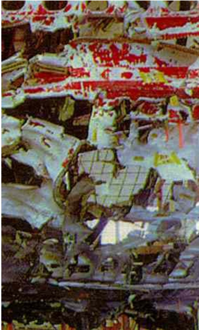
Right side of plane, aft midspan latch of forward cargo door area revealing outward, petal shaped rupture at aft midspan latch and red paint smears.
